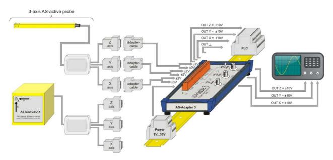
The AS-Adapter 3 offers three measurement channels in a single device. Hence, for the three probe connectors of the single axes only one AS-Adapter 3 is required.
